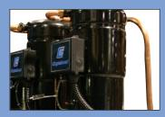
Single or tandem high efficiency scroll compressors
