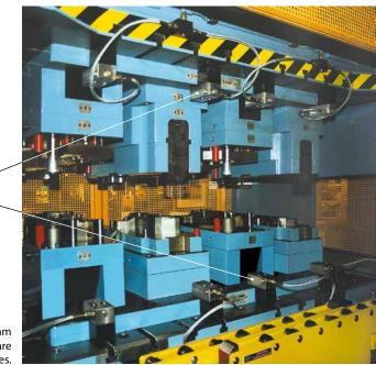
Sliding clamps fastened to bed and ram of a double column press. Dies are entered from the front using consoles.
